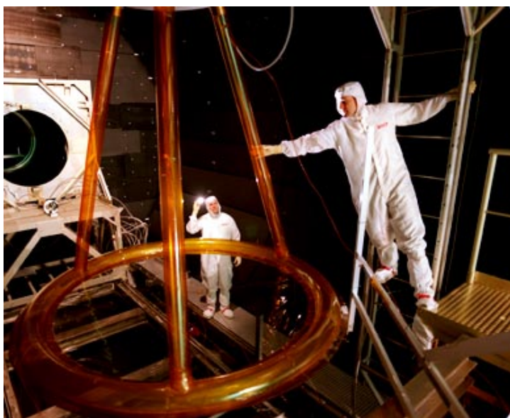
A solar thermal propulsion system that could significantly reduce weight, complexity and cost while boosting performance over current, conventional upper stages is being tested in the Marshall Center's X-ray Calibration Facility. The technology development project — known as Shooting Star — features a 6-foot-wide, thin film lens supported by an inflatable frame. The tests are being conducted in a stainless steel vacuum chamber. The solar thermal propulsion efforts are managed by Marshall's Advanced Space Transportation Program.
