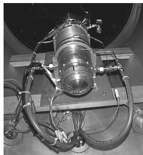
FIGURE 10. RG-350 Stirling Convertor.
