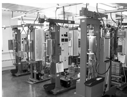
FIGURE 2. IN718 Creep Testing at NASA Glenn.
