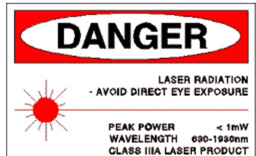
Determine the maximum power density, or intensity, lasers produce when workers are exposed to laser beams. Based on this knowledge, select lenses that protect against the maximum intensity. The selection of laser protection should depend upon the lasers in use and the operating conditions. Workers with exposure to laser beams must be furnished suitable laser protection. [1926.102(b)(2)]
