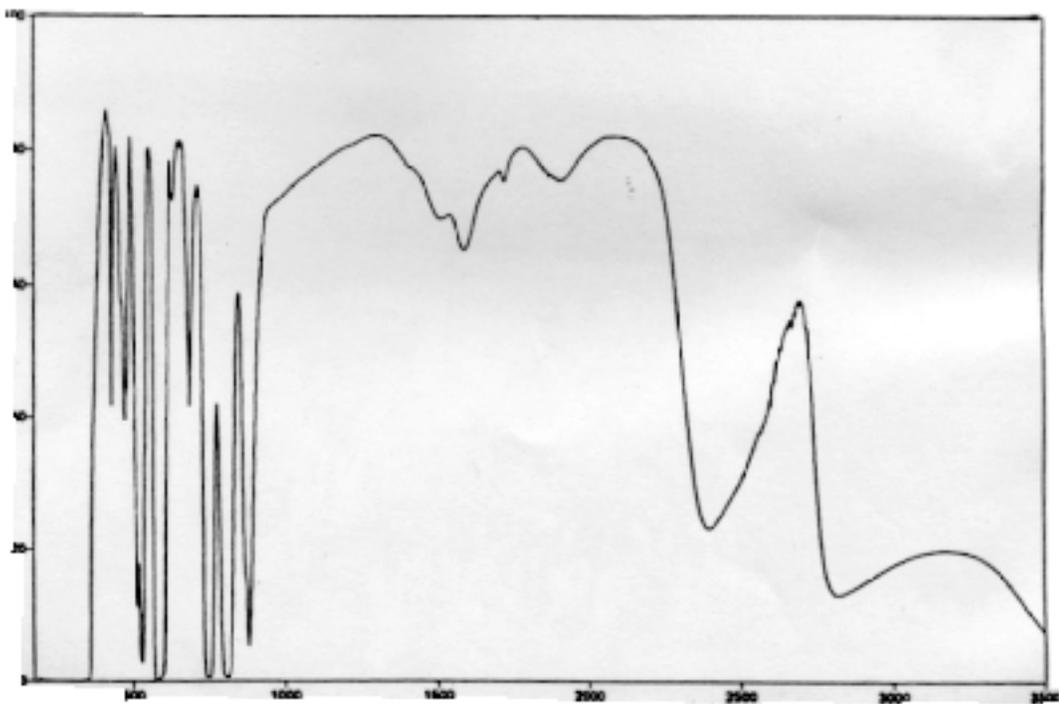
Transmittance / Nanometers **Protective eyewear having high UV, VIS, Blue, and IR transmittance**
