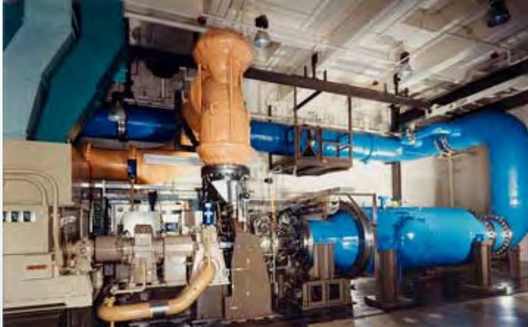
*Upgraded CE-18 high speed compressor test cell*
