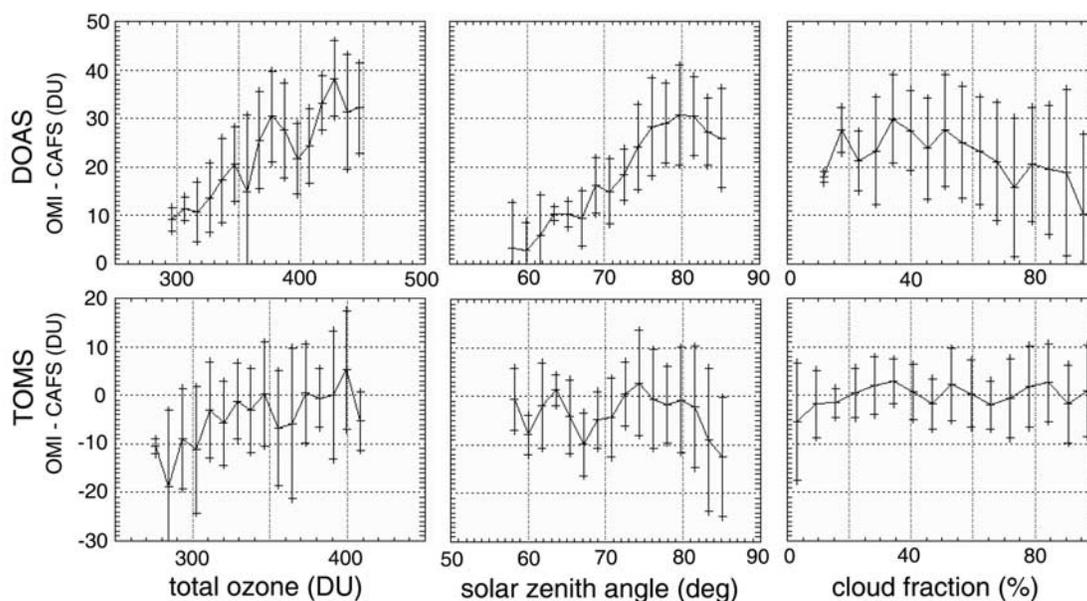
**Figure 8.** The OMI-CAFS total column ozone difference plotted as a function of OMI ozone (left), solar zenith angle (center) and cloud fraction (right). Data averaged from all Polar AVE high-latitude flights. Upper and lower rows depict results using OMI DOAS and OMI TOMS, respectively.
