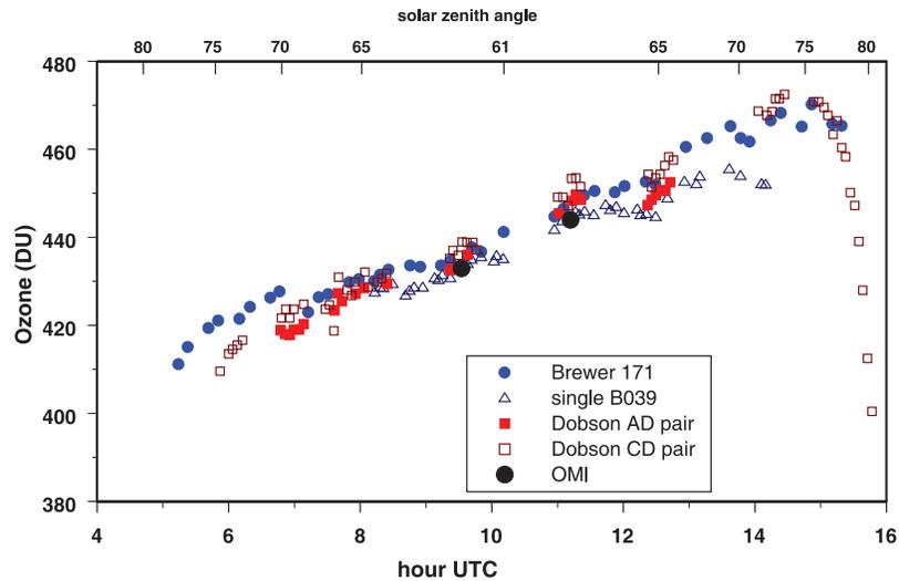
**Figure 9.** Preliminary comparisons from one day during the SAUNA campaign, 5 April 2006. Comparison for Dobson AD observations, Dobson CD, single Brewer (B39), and double Brewer (B171). Two OMI overpass observations are also shown.
