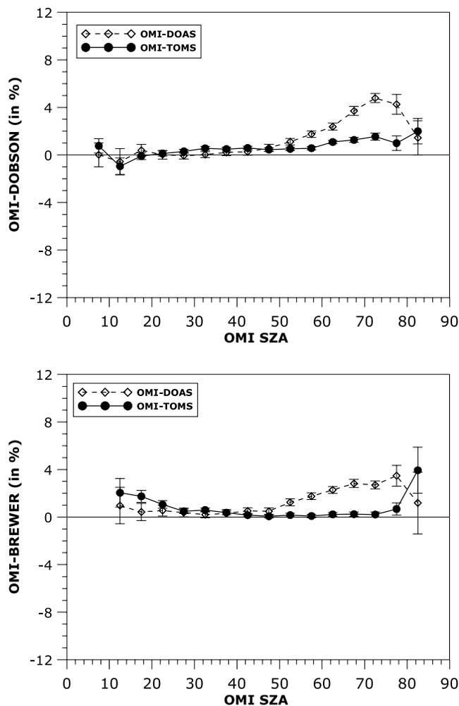
**Figure 3.** Mean relative differences between satellite (OMI-TOMS and OMI-DOAS) and ground-based total ozone data, plotted separately for (top) Dobson and (bottom) Brewer instruments, as a function of the ground pixel solar zenith angle. The error bars depict the two standard errors on the mean.
