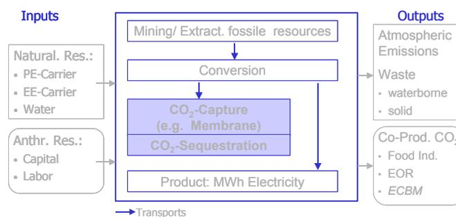
Fig. 6a: Aggregated process chain for electricity production including CO<sub>2</sub>-sequestration (i.e. post-combustion)
