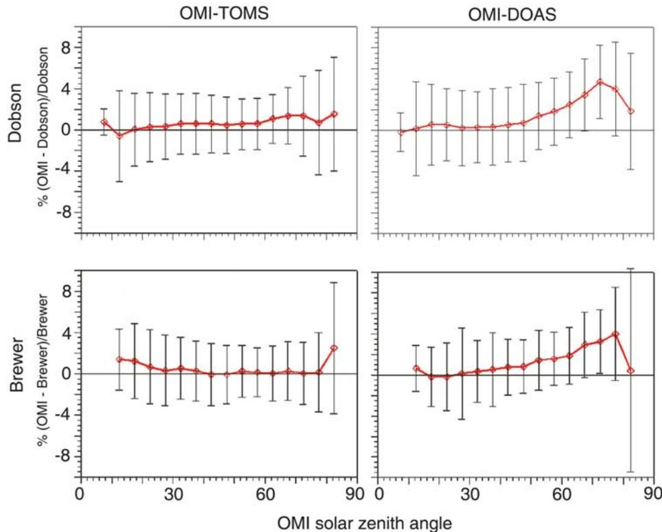
**Figure 7.** Mean relative differences between satellite and ground-based total ozone data, plotted separately for OMI-TOMS and OMI-DOAS (left and right) for Dobson and Brewer instruments (top and bottom), as a function of the satellite solar zenith angle at the ground pixel.
