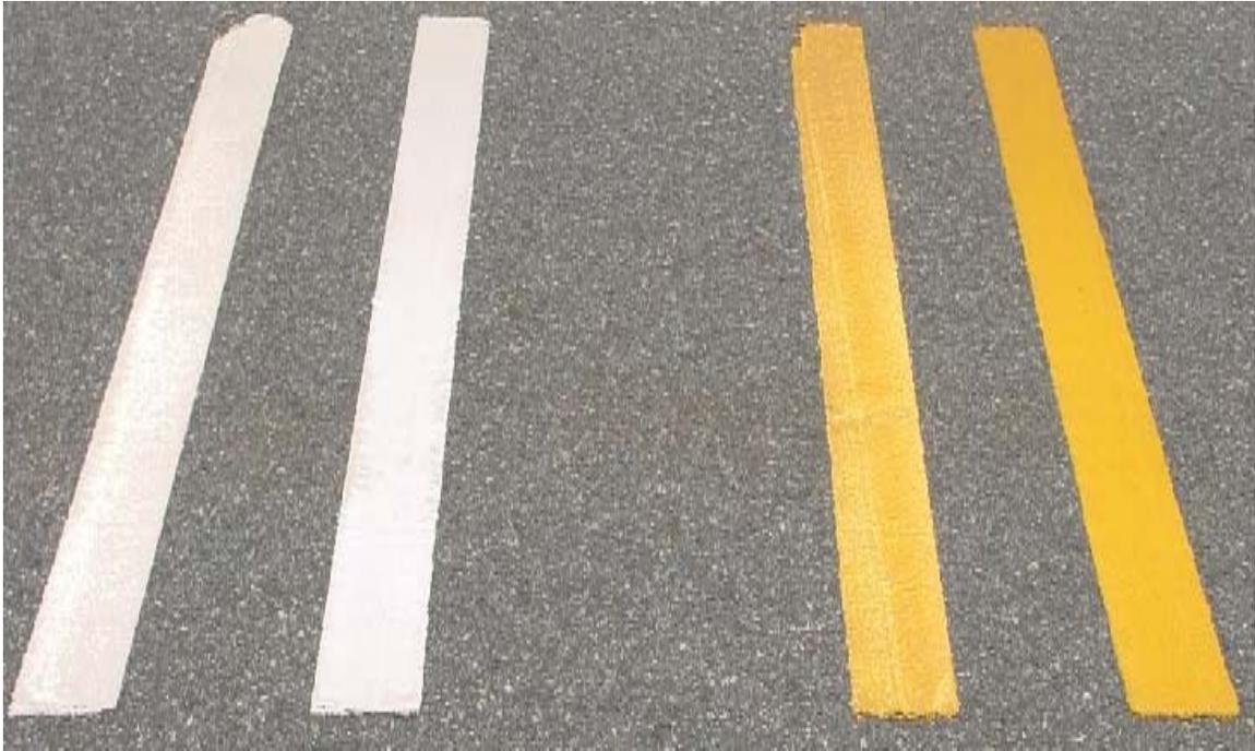
FIGURE 1. POLYESTER MARKING MATERIAL ON ASPHALT WITH TYPE I AND TYPE III BEADS
