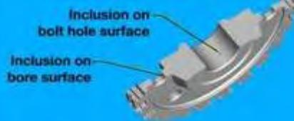
Calculation of Max Principal Stress for a Turboshaft HP Turbine Disk
