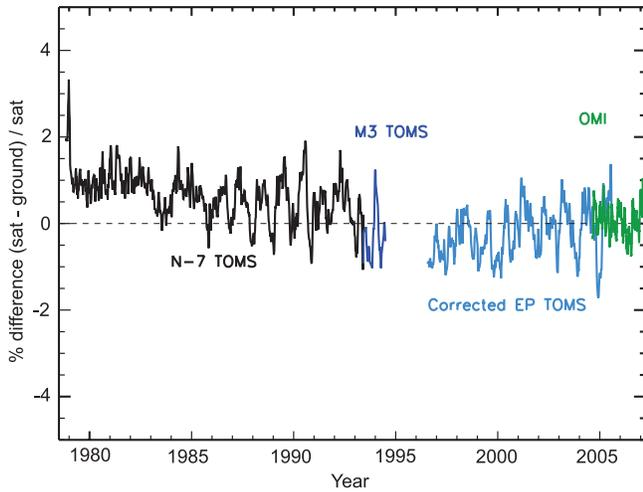
**Figure 2.** OMI ozone in the context of the Nimbus 7 TOMS and Earth Probe TOMS time series. All compared to an ensemble of 30 Northern Hemisphere Dobson stations that have coverage over the 26 year period.
