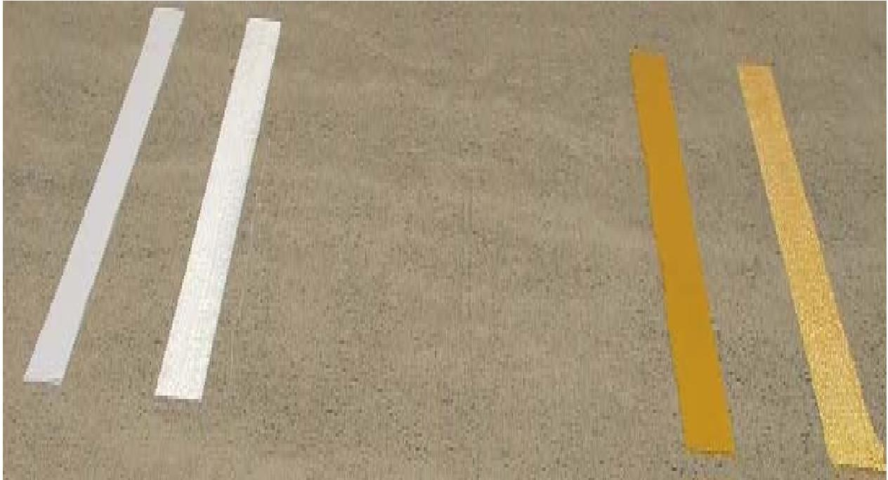
FIGURE 3. POLYESTER MARKING MATERIAL ON AGED PORTLAND CEMENT CONCRETE WITH TYPE I AND TYPE III BEADS
