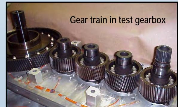
Gear train in test gearbox
