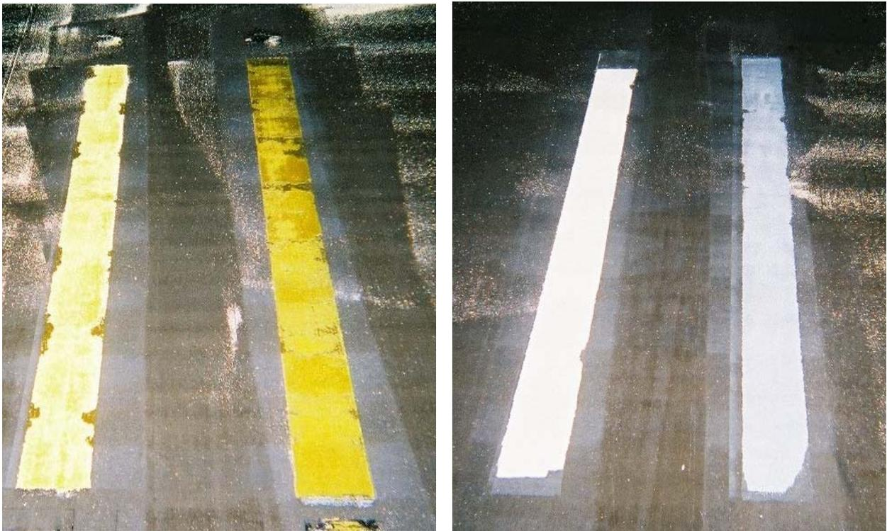
FIGURE 4. POLYESTER MARKING MATERIAL ON NEW PORTLAND CEMENT CONCRETE WITH TYPE I AND TYPE III BEADS
