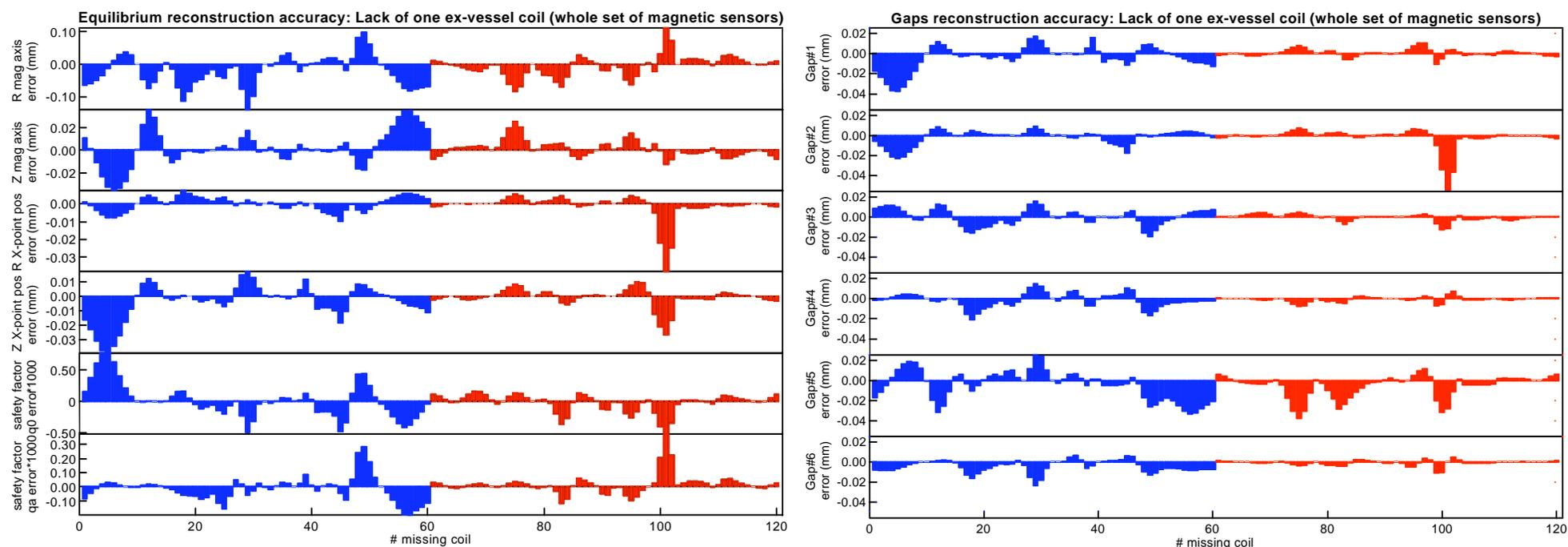
Simulation with all sensors (in-vessel coils, divertor, flux loops and ex-vessel coils). Error due to suppression of one ex-vessel coil assessed: **blue tangential** (1-60), **red radial** (61-120)
