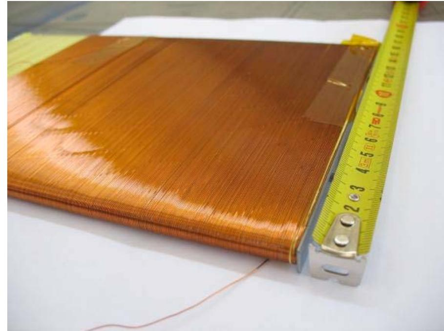
**Prototype of the ex-vessel tangential coil** located in area of large VV curvature.
