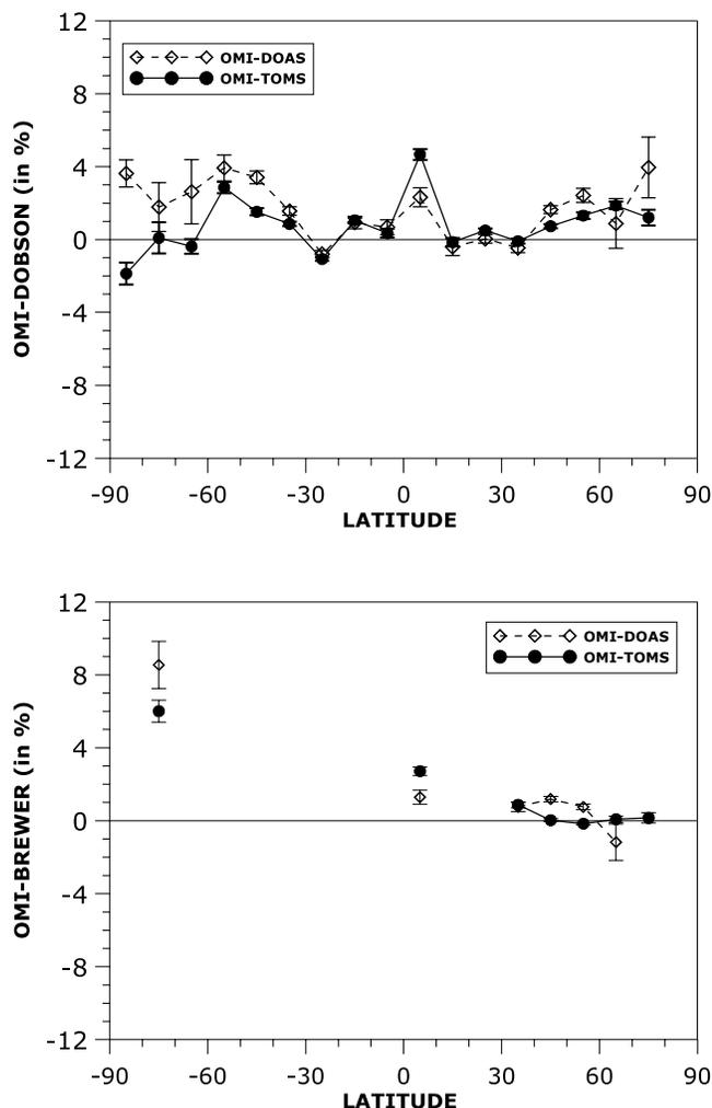
**Figure 1.** Mean relative differences between OMI satellite (OMI-TOMS and OMI-DOAS) and ground-based total ozone data, plotted separately for (top) Dobson and (bottom) Brewer instruments, as a function of the ground pixel/station latitude. The error bars depict two standard errors on the mean.
