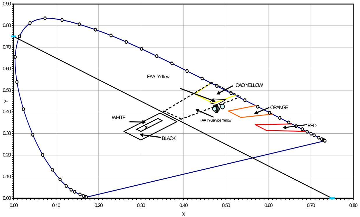
FIGURE A-10. COLOR READINGS (YELLOW) TYPE III BEADS ON AGED CONCRETE
