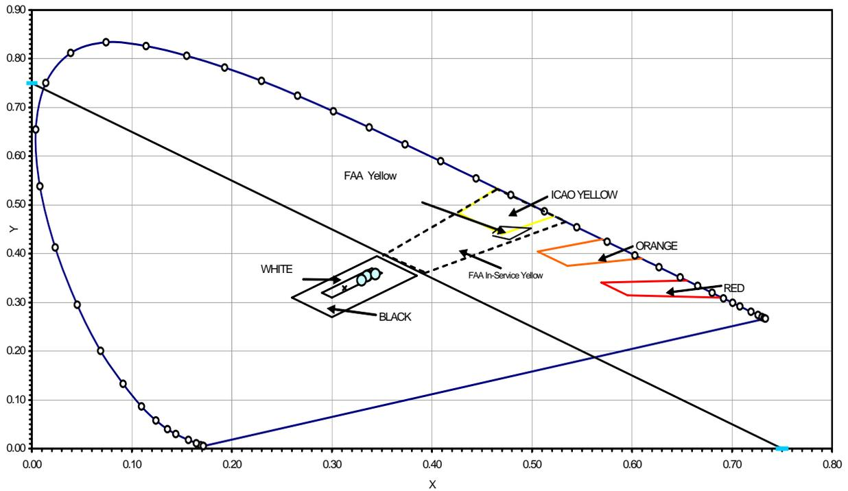
FIGURE A-5. COLOR READINGS (WHITE) CENTERLINE TYPE I ON ASPHALT
