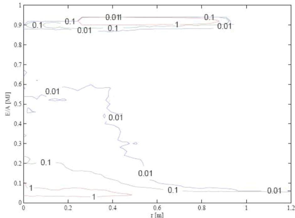
Ratio  $f_{3\text{He}}/f_{\alpha}$  integrated over entire plasma as a function of normalized energy  $E/A$  for 16 MW RF power and a scan of  $^3\text{He}$  concentrations.
