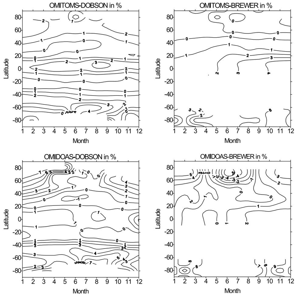
**Figure 2.** Monthly mean relative differences between satellite and ground-based total ozone data, plotted separately for OMI-TOMS and OMI-DOAS in rows and for Brewer and Dobson instruments in columns. OMI data incorporated cover the whole time period 2005–2006 for OMI-TOMS and the whole 2006 for OMI-DOAS.
