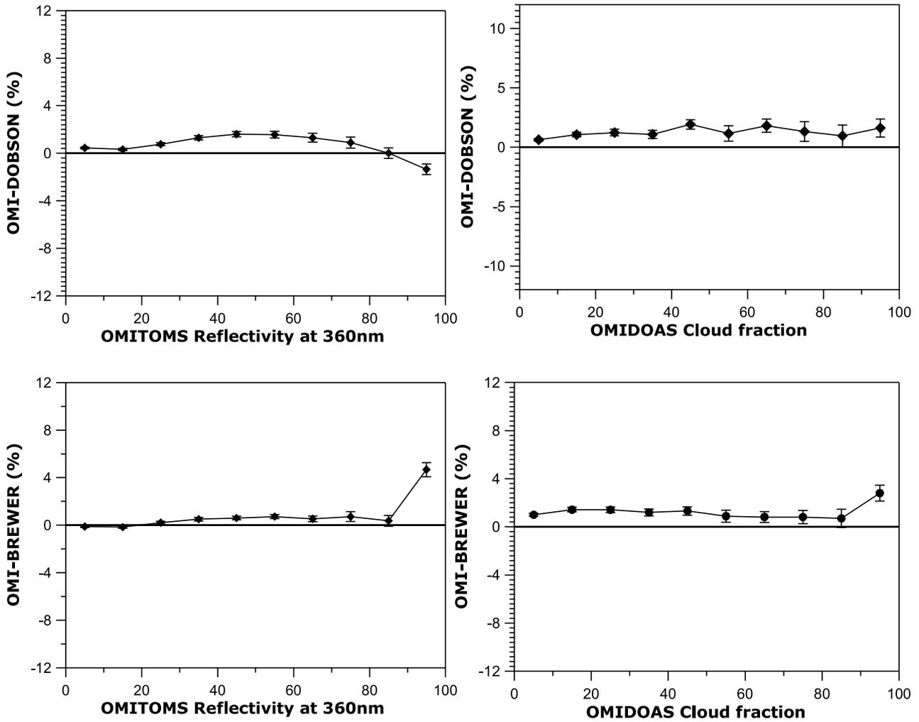
**Figure 4.** (left) Relative difference between OMI-TOMS and ground-based total ozone as a function of the OMI reflectivity data at 360 nm. (right) Relative difference between OMI-DOAS and ground-based total ozone as a function of OMI-DOAS determined cloud fraction. The error bars depict two standard errors on the mean.
