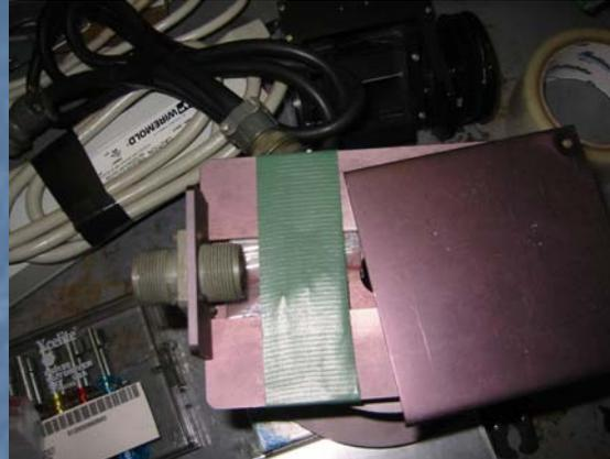
Tape down any loose parts, like the shield on the lamp holder
