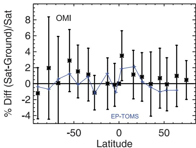
**Figure 3.** The latitude dependence of OMI-TOMS from a comparison with 93 Dobson and Brewer stations worldwide. Average OMI differences from ground stations are plotted for  $10^\circ$  zones with standard deviations. A similar comparison with EP TOMS for the period 1996–2001 (shown in blue) is plotted without standard deviations for clarity.
