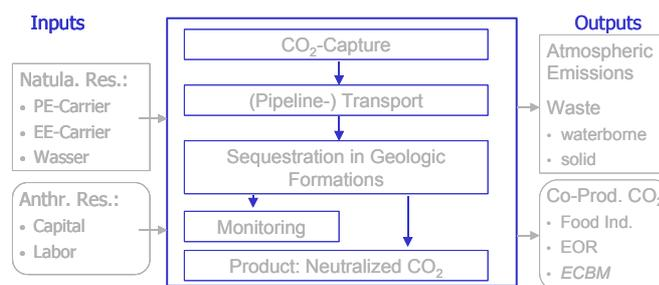
Fig. 6b: Process chain for the part of CO<sub>2</sub>-sequestration (i.e. post-combustion)
