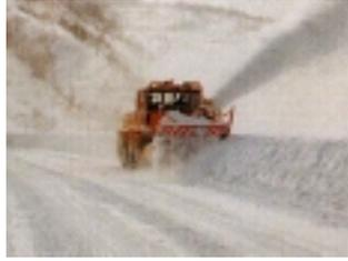
Photograph 2. Rotary Snow Remover Removing Snow
