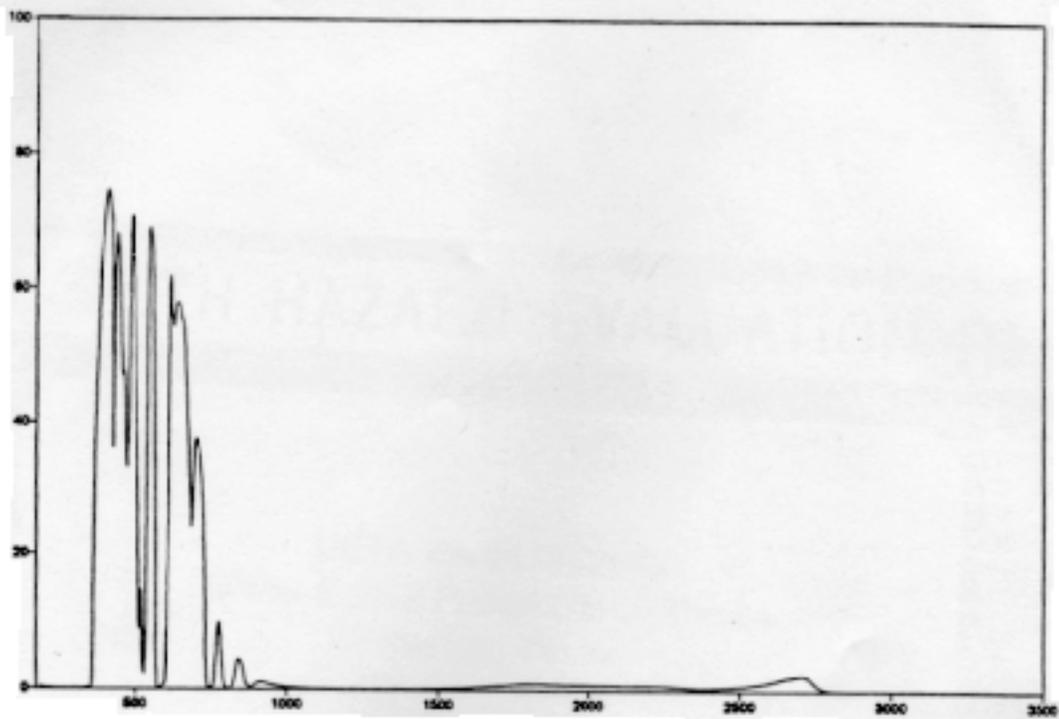
Transmittance / Nanometers **Protective eyewear having high UV, VIS, and Blue light transmittance**
