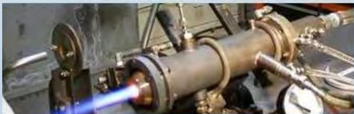
Erosion Test Rig & Axisymmetric CFD of bumer rig flame
