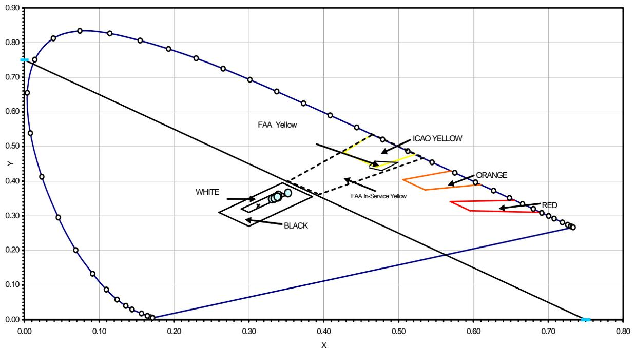
FIGURE A-3. COLOR READINGS (WHITE) TYPE III BEADS ON ASPHALT
