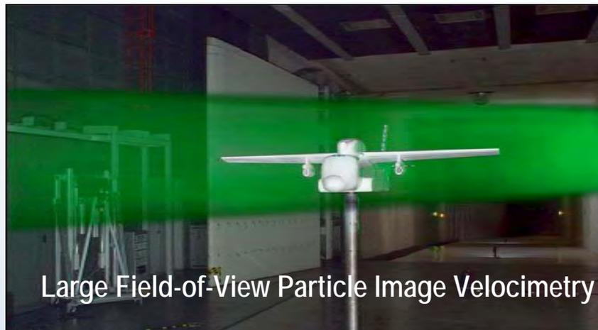
Large Field-of-View Particle Image Velocimetry
