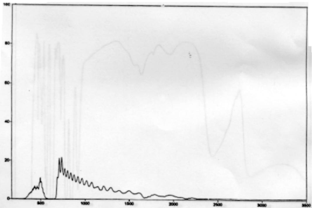
Transmittance / Nanometers **Protective eyewear having low UV and Blue transmittance**
