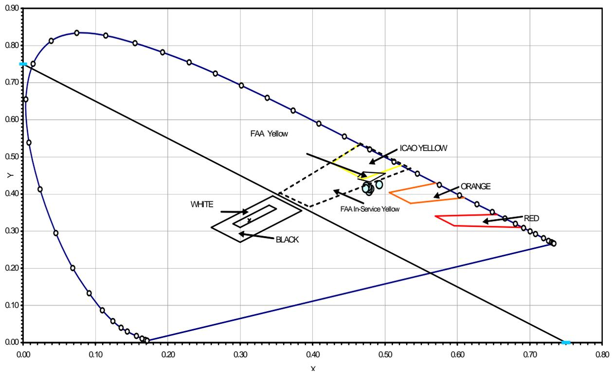
FIGURE 5. SAMPLE COLOR READINGS (YELLOW) TYPE III BEADS ON AGED CONCRETE
