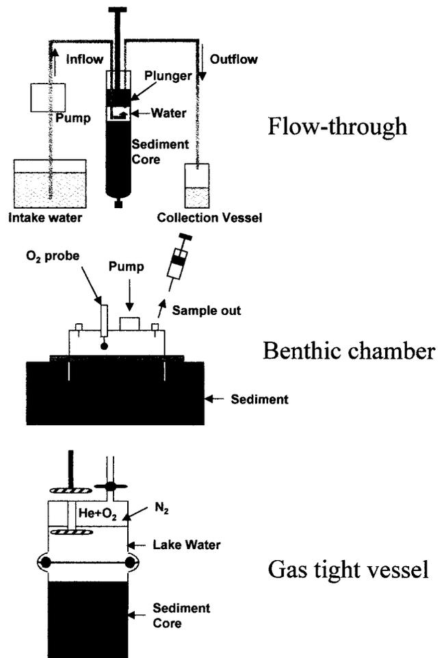
FIG. 2. Schematic diagram of three experimental systems for measuring sediment-water nitrogen fluxes.
