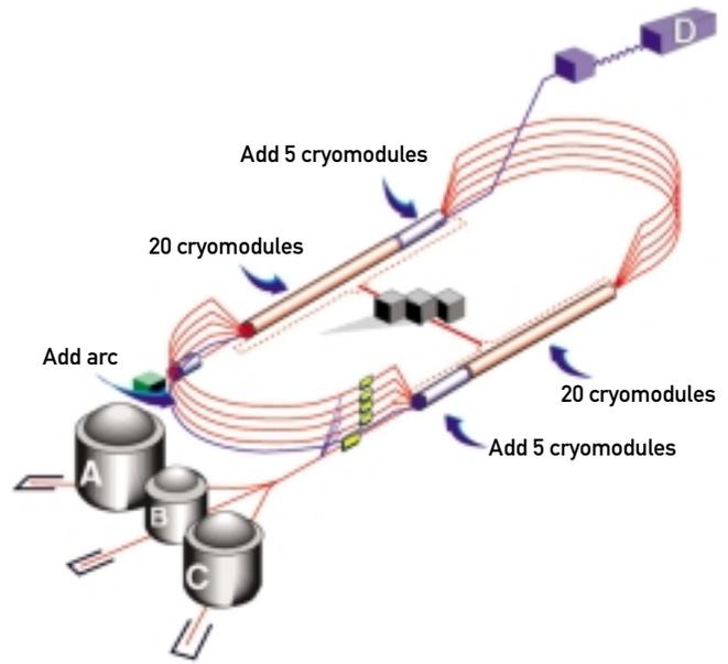
**Figure 5.3.** Elements of the CEBAF upgrade. Increasing the beam energy at CEBAF from 6 to 12 GeV requires upgrades in four areas: (i) additional accelerating power, (ii) stronger magnets in the recirculation arcs, (iii) an upgraded cryoplant, and (iv) one additional recirculation arc. The higher-energy electrons can be directed to a new experimental area, Hall D.
