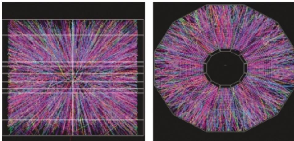
**Figure 2.15.** Golden glow. A central gold-gold event as seen in the STAR detector at RHIC. The side view and end view of the time-projection chamber are shown. Each colored radial line emanating from the center corresponds to the track of a particle produced in the collision. Such a central collision typically produces about 6000 particles.
