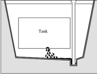
When installed and operated according to the manufacturer's specifications, secondary containment with interstitial monitoring meets the federal leak detection requirements for USTs. Operation of the monitoring device at least once each month fulfills the requirements for the life of the tank. Secondary containment with interstitial monitoring can also be used to detect leaks from piping (see the section on leak detection for piping starting on page 22).
