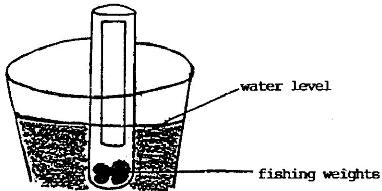
4. Holding the test tube gently against the cup, mark the water level on the tape with a marking pen.
