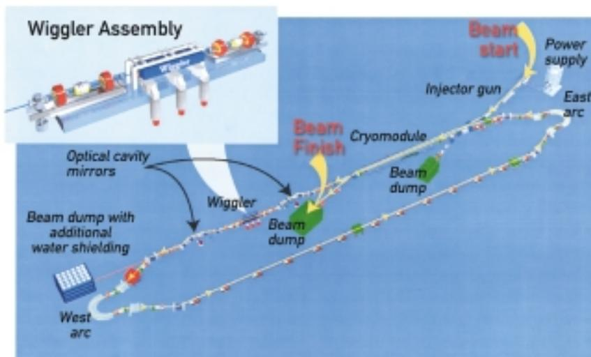
**Figure 4.11.** A world-record tunable laser. Free electron lasers work by coaxing coherent radiation from electrons by subjecting them to the alternating magnetic fields of a wiggler. As they “wobble,” the electrons emit light, whose wavelength can be tuned by varying the wiggler gap through which they pass. This schematic shows the Jefferson Lab FEL, which has achieved world-record intensities for a tunable laser.
