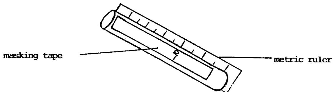
7. Write numbers less than 10 (9,8,7,etc.) next to the marks **above** the 10 mark. Put numbers greater than 10 (11,12,13,etc.) next to the marks **below** the 10 mark.
