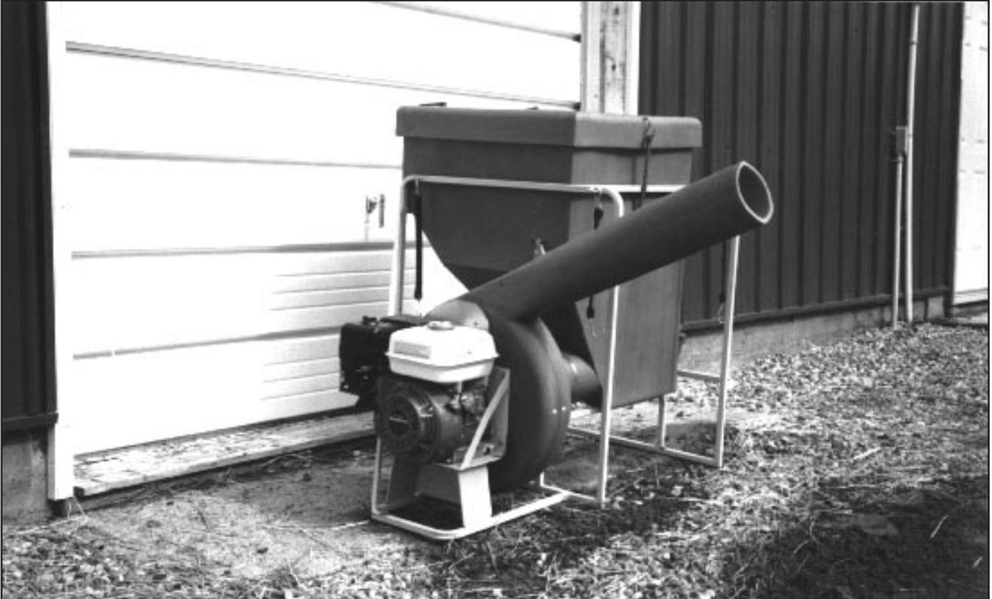
(fig. II.19–1), measure swath width while the spreader is actually mounted on the vehicle and preferably under the same conditions that you will experience during bait applications. Swath width measurement and actual bait applications should be done by traveling directly into or against the prevailing wind.
