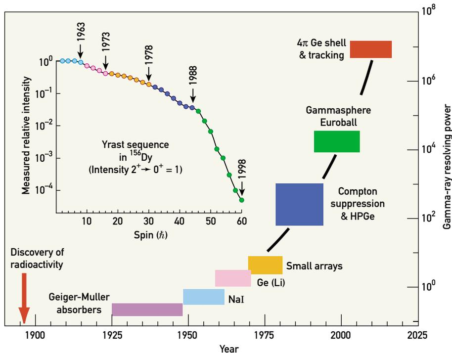
**Figure 5.4.** Evolution of gamma-ray detection technology. The large gain provided by a  $4\pi$  tracking array, such as GRETA, is clearly shown. The calculated gamma-ray resolving power is a measure of the ability to observe the faint emissions from rare and exotic nuclear states. This is illustrated in the top left-hand insert, which indicates the strong inverse relationship between resolving power and the experimental limit for observing excited states in a typical rare-earth nucleus.
